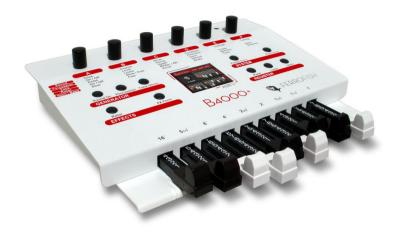
The **B4000+** can receive MIDI either with the implemented MIDI connectors or receive and transmit MIDI via the USB connector.
