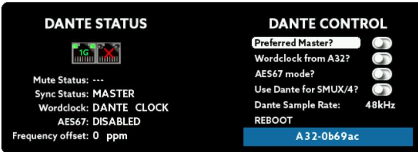
**Ethernet Ports:** Shows the status and speed of the Ethernet ports in use (Pri/Sec).
