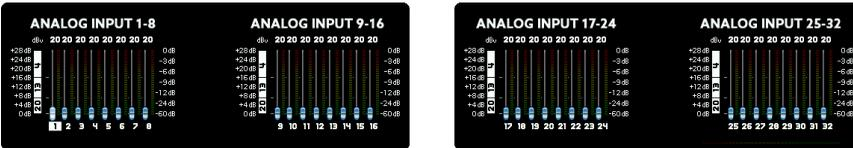
The number above the fader shows the maximum level (dBu), which the input can handle. When the fader is set to 20, like shown in the picture above, the input can handle a maximum input level of +20dBu. Avoid exceeding this maximum level to prevent digital clipping.
