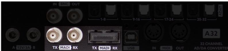
Use either optical fiber cables (SC connectors) or coaxial cable with an impedance of 75 ohms (BNC connectors) for MADI.
