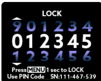
After entering the correct number, hold down the MENU button for a few seconds to activate the lock.
