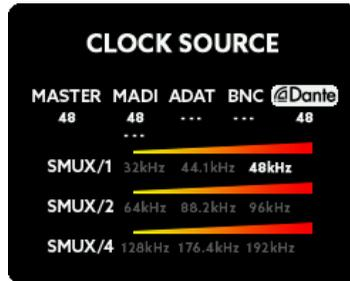
The numbers below the labels show the internally generated clock as Master or the measured external sample rate. If no sample rate is detected, „---“ will be displayed.
