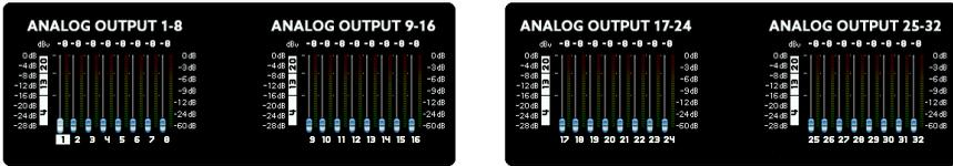
If you select one of the three reference levels exactly, the digital signal will be converted 1:1 to analog. However, if you select a value in between these reference levels, the DSP will calculate the optimal combination between analog and digital levelling. For example, if you select +12dBu the analog output will be switched to +13dBu and the digital signal will be attenuated by 1dB to reach the +12dBu output level.
