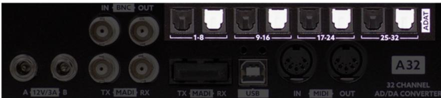
The ADAT ports are switched off when using the SMUX/4 mode.
